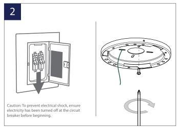
1. Attach the mounting bracket to the outlet box with two screws and washers provided. Make sure the bracket is tight and secured. For UL Junction box installation, use **A** parts.
